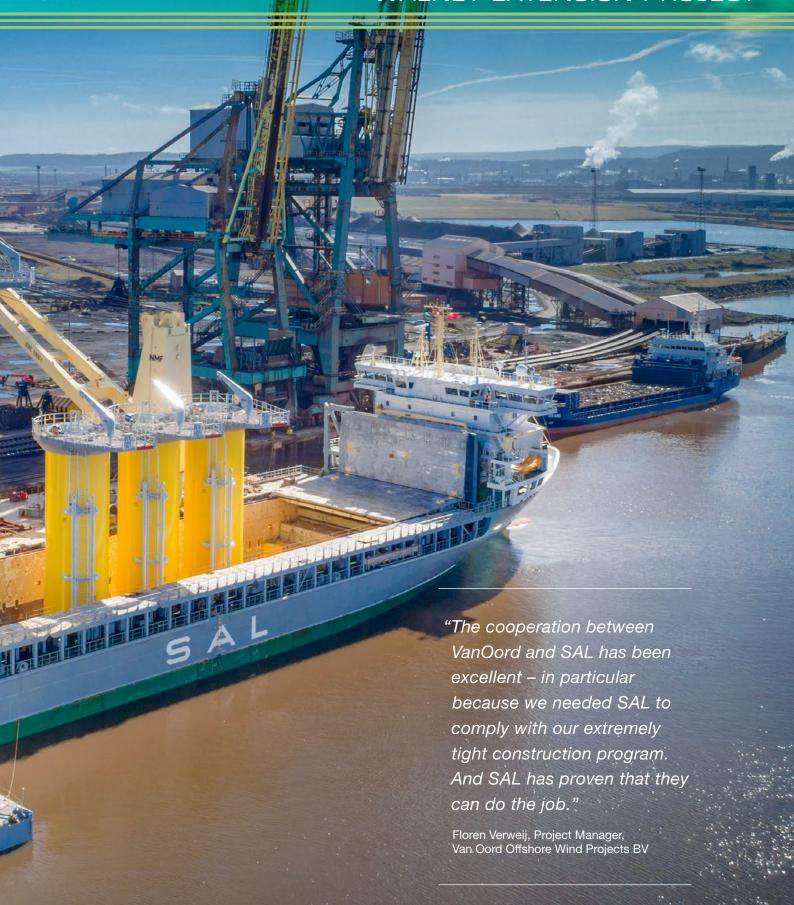
e continue the story on our long-term project Walney Extension. One major requirement for a successful performance of the project is the flexibility to change rapidly between two different cargo settings. The Monopiles (MPs) have been lifted and transported in a horizontal position whereas the Transition Pieces (TPs) need to stay upright when moved. >>
