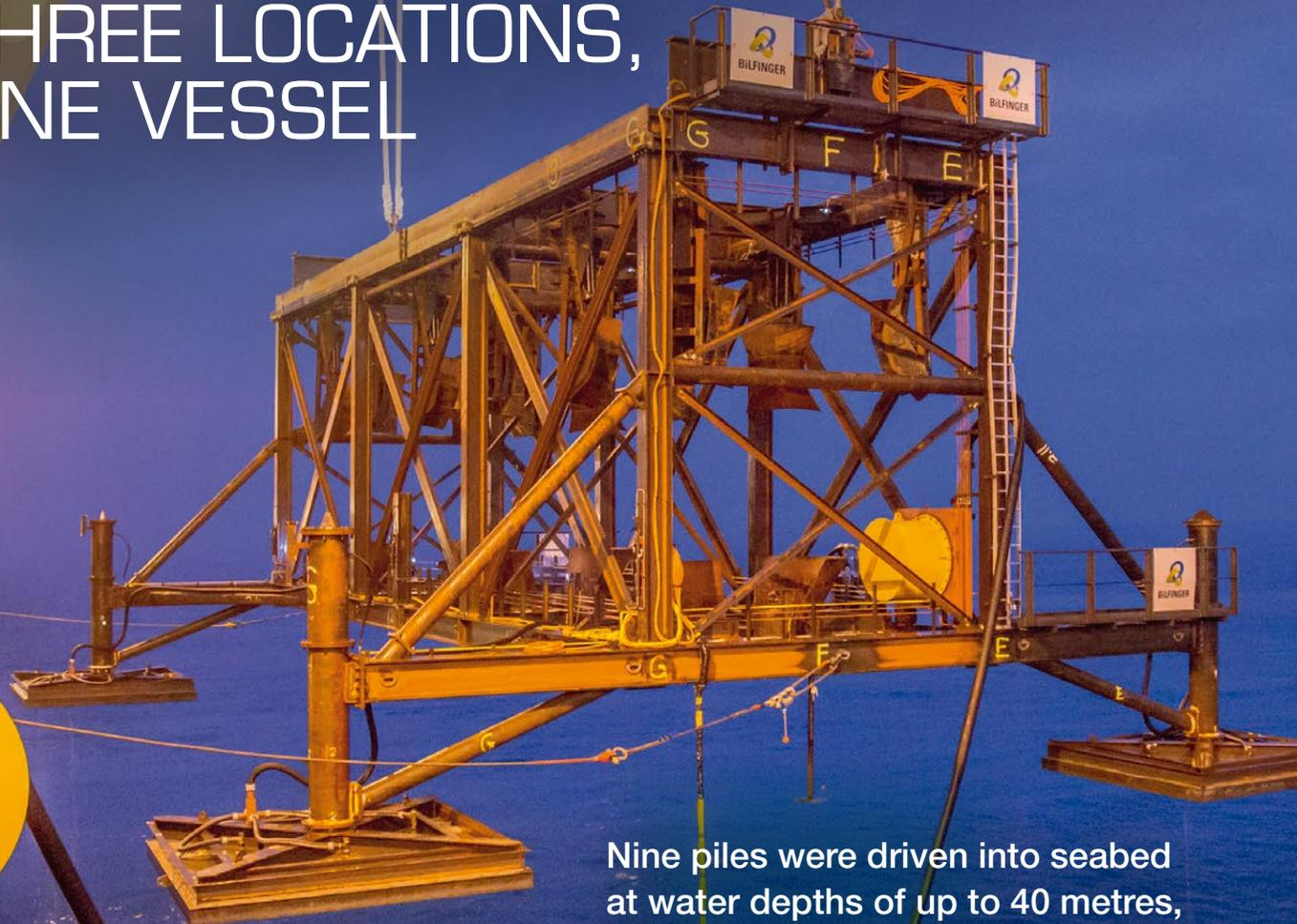
Nine piles were driven into seabed at water depths of up to 40 metres, followed by strike and pull out tests. Once again MV Lone served as perfect project platform.
